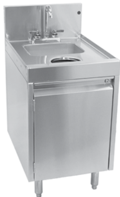
SWB-18-DW - Includes a sink with faucet and lift-out perforated plastic wet waste strainer, dry waste chute and cabinet base with hinged access door for storing a trash receptacle. A stainless (DWC) or plastic (03005391) trash receptacle is offered as a separate accessory.
