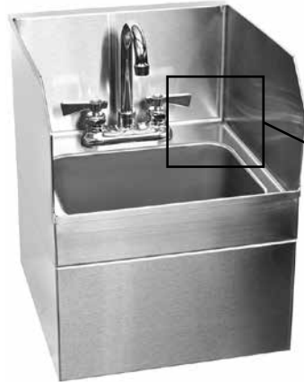
Model WHS-14-S featuring integral side splashes, radius work surface corners for easy cleaning and a front lip to contain splashes
