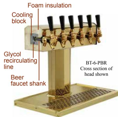
Properly chilling the beer faucets prevents intermittent foaming problems. Each Glastender beer tower includes a special glycol-chilled cold plate assembly that envelops the faucet shanks to keep the beer faucets cold.
