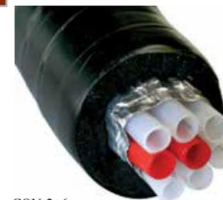
Glastender line sets use special barrier tubing to resist build-up and prevent flavor transfer. The beer lines surround super-chilled glycol lines and are foil wrapped and insulated to maximize cooling. A PVC vapor barrier outside wrap protects the line set from humidity, tears, and abrasions.
