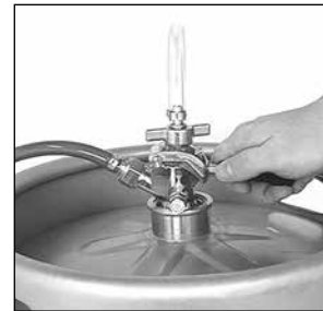
Pull the handle out and push it down to the locked position, which activates the pressure and beer lines. You are now ready to draw beer.
