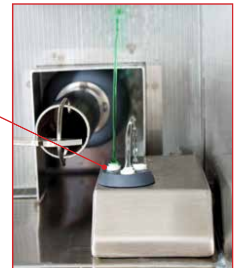
Chemical fill is easily visible by sliding the cover open during the fill portion of the wash and rinse cycles.
