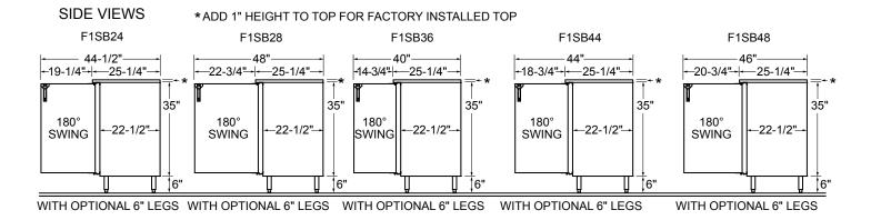
Note: Available with compressor left or right. Compressor left model shown.
