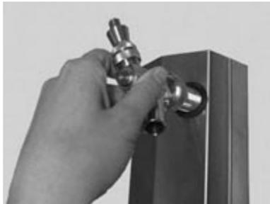
12. This step is for remote cooled towers. Put 3 drops of Loctite® into each threaded cold plate hole. Then, tightly screw faucet and shank into the column. If the faucet angle is wrong, loosen nut with spanner wrench, leaving the shank in place. Adjust the faucet angle and tighten nut.
