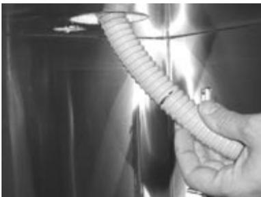
15. This final step is for air cooled towers only. The keg cooler should include a blower hose for cooling the tower. Place the open end of the blower hose inside the column from inside the cooler up to the marked position.
