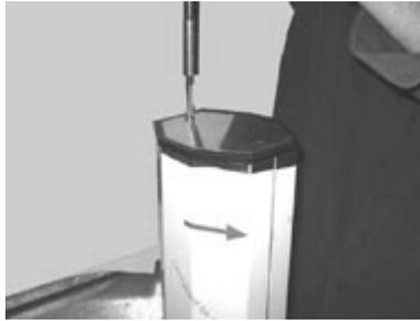
2. Remove the two #10-32x1-1/4" phillips truss head s/s machine screws and column top plate. Slide up the column skin to expose the mounting holes.
