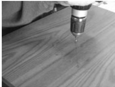
5. Drill all holes using a 1/8" drill bit.
