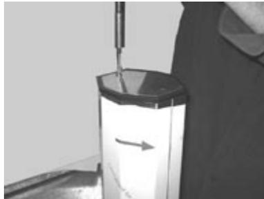
13. Mount the column top plate to the column stiffener with the two #10-32x1-1/4" phillips truss head s/s machine screws provided.
