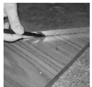
4. Using a straight edge and the four column stiffener mounting holes, mark the center of the beer line hole.
