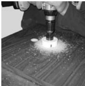
7. Drill the beer line hole(s) and drain hole to 1/4". Finish the drain hole at 1-1/2", and the beer line hole at 3-1/4" using an appropriately sized hole saw.
