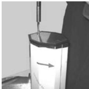
2. Remove the two #10-32x1-1/4" phillips truss head s/s machine screws and the column top plate. Remove the column skin from the column stiffener.
