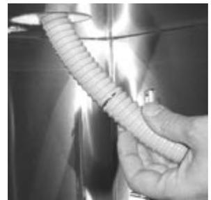
18. This final step is for air cooled towers only. The keg cooler should include a blower hose for cooling the tower. Place the open end of the blower hose inside the column from inside the cooler up to the marked position.
