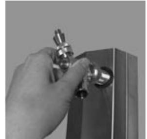
15. This step is for remote cooled towers. Put three drops of Loctite® into each threaded cold plate hole. Then, tightly screw faucet and shank into the column. If the faucet angle is wrong, loosen nut with spanner wrench, leaving the faucet in place. Adjust faucet angle and tighten nut.
