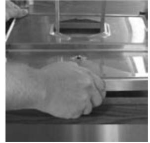
12. Place the drain pan over the column stiffener and base plate.
