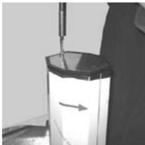
16. Mount the column top plate with the two #10-32x1-1/4" phillips truss head s/s machine screws provided.
