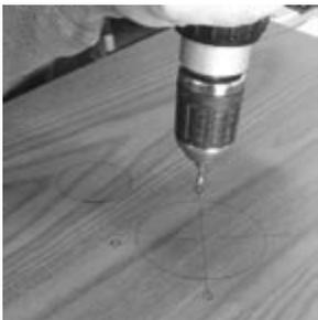
5. Drill all holes using a 1/8" drill bit.
