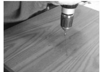
3. Drill all holes using a 1/8" drill bit.
