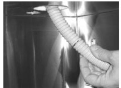
14. This final step is for air cooled towers only. The keg cooler should include a blower hose for cooling the tower. Place the open end of the blower hose inside the column from inside the cooler up to the marked position.
