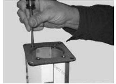
11. Mount the top head plate to the column stiffener with the four #10-32x5/8" phillips flat head s/s machine screws provided.
