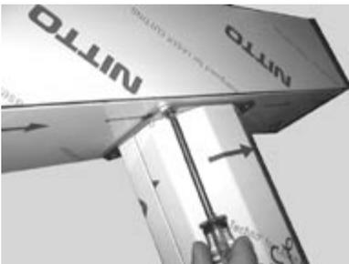
12. Mount the tower head to the column by sliding the line set through the column and securing the head to the top head plate with the four 1/4"-20x1/2" phillips flat head screws provided.
