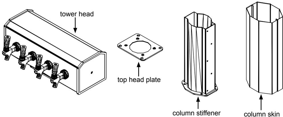
NOTE If your Beer Tower was partially installed in the factory, start with installation step #8.
