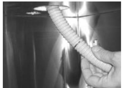
17. This final step is for air cooled towers only. The keg cooler should include a blower hose for cooling the tower. Place the open end of the blower hose inside the column from inside the cooler up to the marked position.
