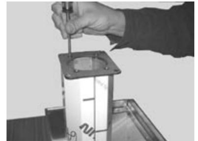
14. Mount top head plate with the four #10-32x5/8" phillips flat head s/s machine screws provided.
