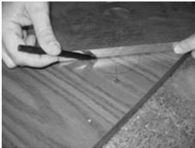
2. Using a straight edge and the four column stiffener mounting holes, mark the center of the beer line hole.
