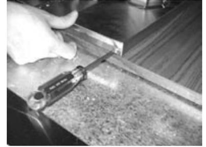
11. Secure the drain pan to the base plate with the four #10-32x1/2" phillips pan head s/s machine screws provided (will be brass screws for brass towers).
