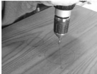
3. Drill all holes using a 1/8" drill bit.
