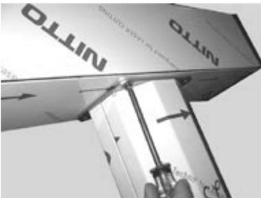
15. Mount the tower head to the column by sliding the line set through the column and securing the head to the top head plate with the four 1/4"-20x1/2" phillips flat head screws provided.
