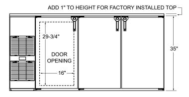
Note: Available with compressor left or right. Compressor left model shown. Use Model Number Key to specify location when ordering.
